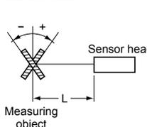
Aluminum vapor deposition surface reflection mirror (0°, ±0.2°)
