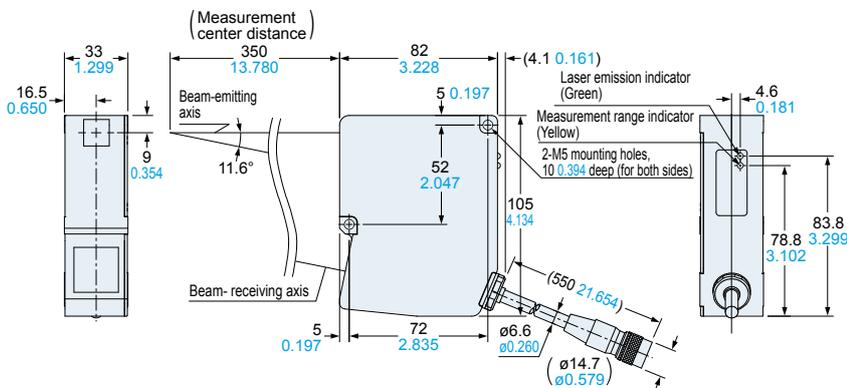
**Setup mode: Specular reflection type**
