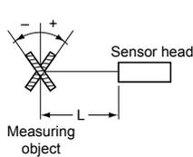
Aluminum vapor deposition surface reflection mirror (0°, ±0.05°)
