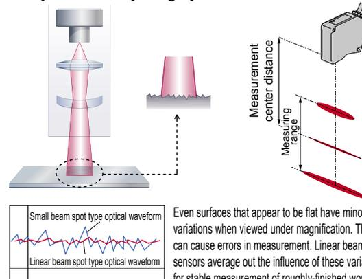
Even surfaces that appear to be flat have minor surface variations when viewed under magnification. These variations can cause errors in measurement. Linear beam spot type sensors average out the influence of these variations, allowing for stable measurement of roughly-finished workpieces.
