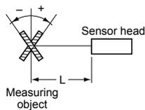
Aluminum vapor deposition surface reflection mirror (0°, ±0.2°)
