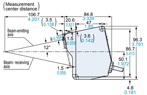
**HL-G1** Note: A beam attenuator is not available for IEC/JIS conformed types.
